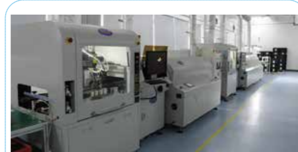
Note: The automatic spraying process of conformal coatings
