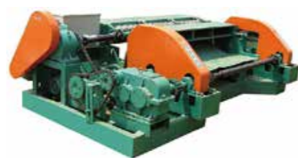
Rotary cutter for the wood processing equipment
