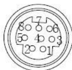
(8 芯 DB 接口) 8-pin DB connector
